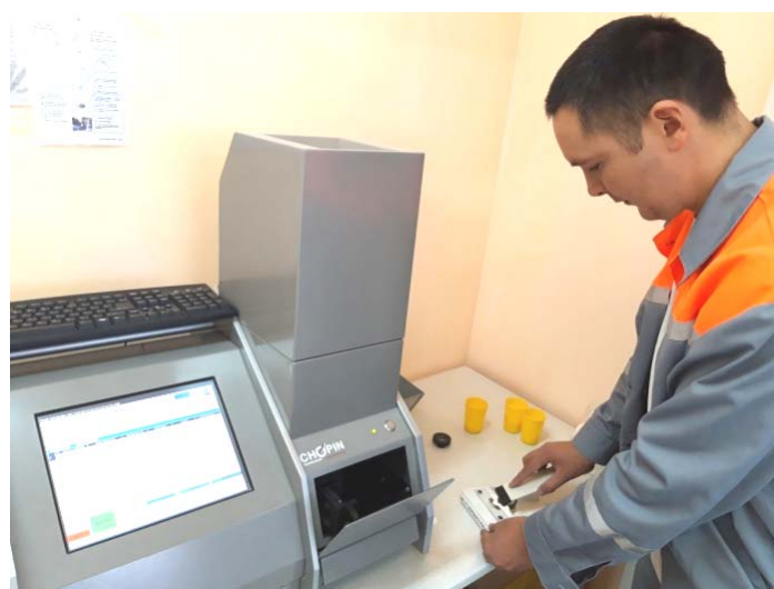
Figure 2 - The process of analyzing the sample of flour on the device INFRANEO
