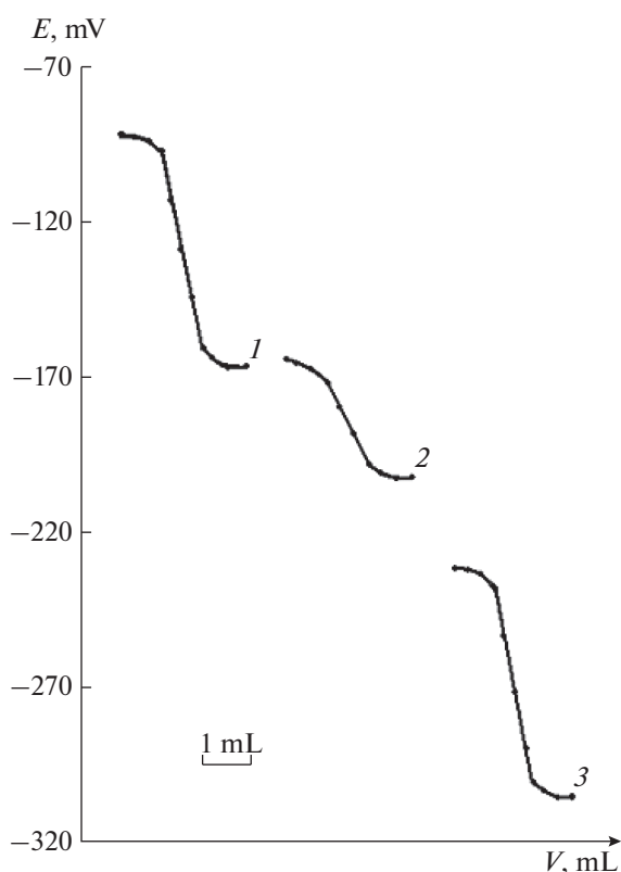
Fig. 4. Curves of potentiometric titration of cadmium ions with a 0.01 M \text{Na}_2\text{S} solution using (1) Cd-SE and GaAs electrodes (2) before modification and (3) after modification.
