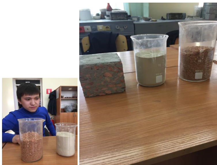
Figure 1. General view of a chemically active filler, thermolitic sand and concrete sample based on them for a pile foundation.
