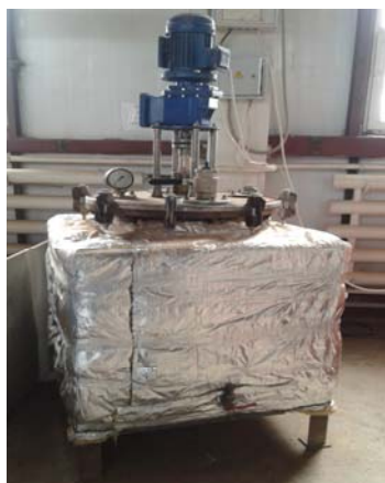
Figure 1 - General view of the reactor for the hydrolysis of horns and hooves
