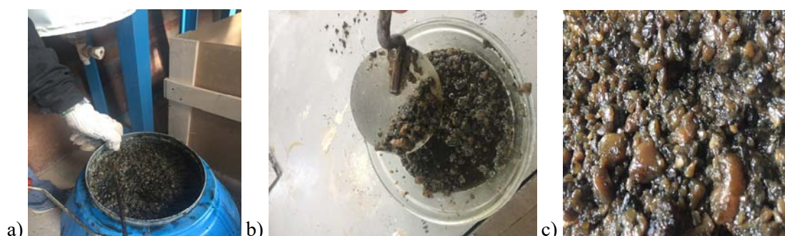
a) the process of separating the liquid part from the solid through a sieve; b) the solid part of the hydrolyzate; c) the solid part of the hydrolyzate under a microscope, x50 magnification
