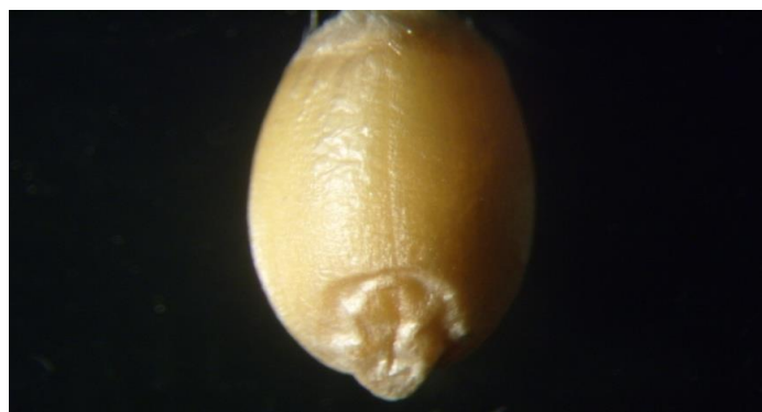
Figure 2. Grain processed by acoustic cavitation during 30 sec. ( \times 4 ).
