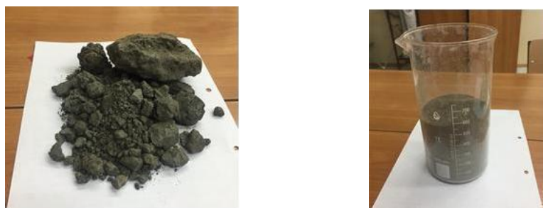
Figure - 1 Montmorillonite clay of the Pogodaevsky deposit, West Kazakhstan region in natural appearance and ground (powder)
