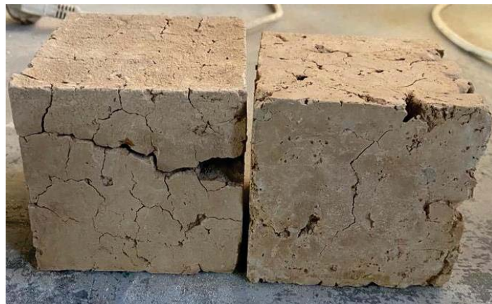
Picture 1 – Ground concrete with the addition of 10% cement
