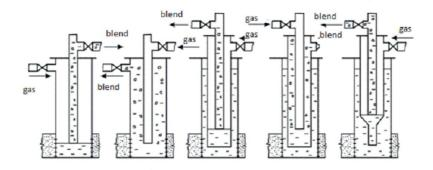
Figure 1 Construction of gas-lift eductors
